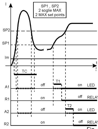
A2) flashes quickly, at the end of T1 (or T2) the led A1 (and/or A2) remains lighted, with FIXED LIGHT, if the overcoming continues to be present. The led A1 (or A2) flashes at LOW FREQUENCY, if the memory started and the overcoming stopped.
